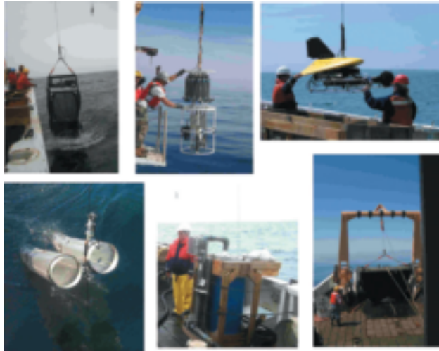
Figure 5. Sampling systems used during the GLOBEC ocean sampling program (clockwise from the upper left): A 1-m 2 Multiple Opening and Closing Net and Environmental Sensing System (MOCNESS), a conductivity-temperature-depth (CTD) profiling instrument with a rosette of bottles to collect water samples, a Video Plankton Recorder (VPR), a large (10-m 2 net opening) MOCNESS system, a pumping system to bring water from depth to the surface for sampling, and a bongo net.
