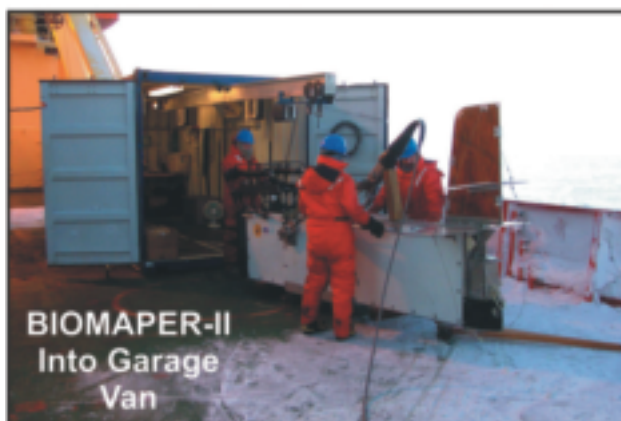
Figure 2. BIOMAPER-II being recovered from a tow between stations 62 and 63 west of Alexander Island on RVIB Nathaniel B. Palmer cruise 0104 (top). The vehicle operates to depths of 300 meters at speeds of 4 to 6 knots. BIOMAPER-II being moved into a heated van for storage after the tow between stations (bottom).
