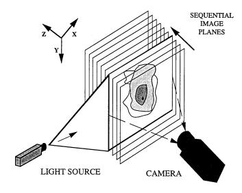
Figure 2. Components of the light stripe imaging system.
