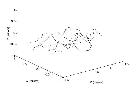
Figure 1. Six target tracks, reconstructed from an FTV sonar image.
